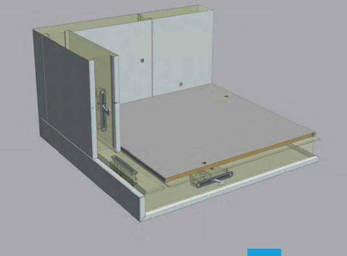
The **ILKA**SYS system makes it possible to produce coldrooms and deep-freeze cells of almost any size in a 300 mm grid. Steps of 100 mm are also possible as an option. This flexibility allows us to adapt our products directly to your local conditions. Upon request, we also manufacture our cells according to your measurements.
